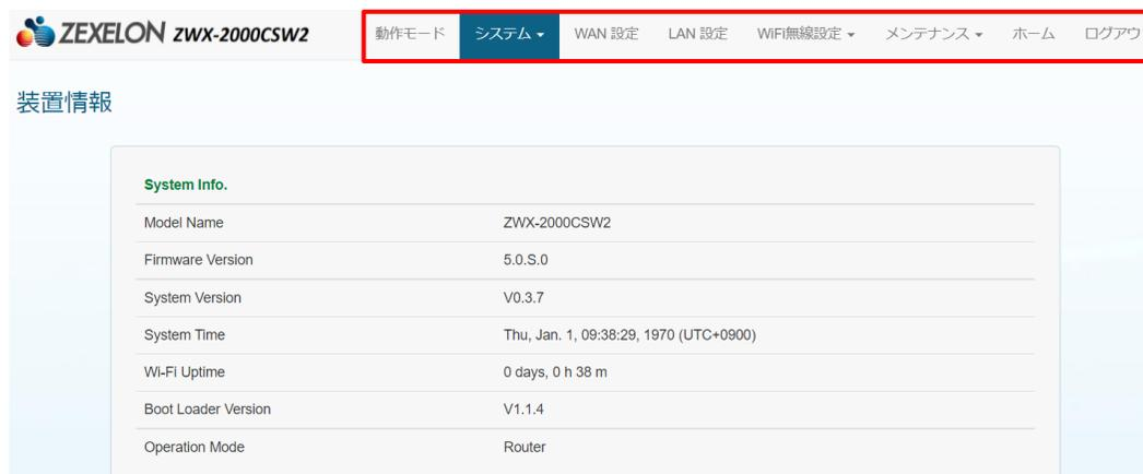
The screenshot shows the web interface for the ZEXELON ZWX-2000CSW2 device. At the top, there is a navigation menu with the following items: 動作モード, システム (highlighted with a red box), WAN 設定, LAN 設定, WiFi無線設定 (with a dropdown arrow), メンテナンス (with a dropdown arrow), ホーム, and ログアウト. Below the menu, the page title is "装置情報" (Device Information). The main content area displays "System Info." with the following details:
